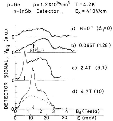
FIG. 4.  $n$ -InSb detector signals as a function of  $B_d$ . The dotted line in (d) indicates spectral response of the detector. Arrows in (c) and (d) indicate the energy position  $\epsilon = \hbar e B / m_1^*$ .
