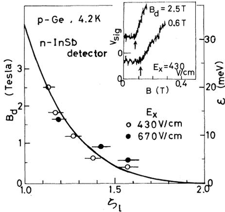
FIG. 3. Kink position  $\zeta_1$  in the  $V_{\text{sig}}$  vs  $B$  curve, taken with  $n$ -InSb detector, as a function of detector magnetic field  $B_d$ . A solid line is drawn according to Eq. (2). Curves of  $V_{\text{sig}}$  vs  $B$  at different  $B_d$  are shown in the inset.
