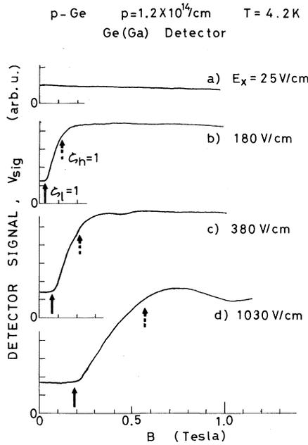
FIG. 1. Ge/Ga detector signals as a function of sample magnetic field  $B$  at different levels of  $E_x$ .
