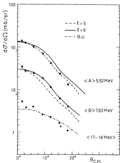
FIG. 2. Angular distributions from the reaction  $^{144}\text{Sm}(\alpha, t)^{145}\text{Eu}$  to high-lying proton states. The centroid energy of the bumps are indicated. Solid and dashed lines are DWBA calculations (bound state, region A; Gamov function, region B) for the indicated  $l$  values. Error bars are statistical errors only. The dot-dashed curve corresponds to the theoretical prediction of the breakup model for the indicated energy bin in region C.
