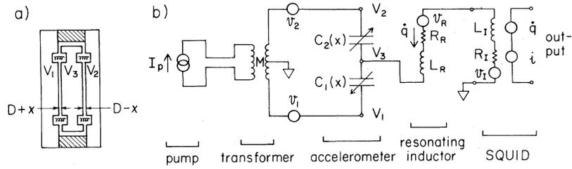
FIG. 1. (a) A schematic diagram of an accelerometer. An impulse applied to the outer plates causes the relative coordinate  $x$  to oscillate. (b) The electrical schematic of the bridge circuit used to sense the motion of  $x$ . Noise generators are labeled with italic letters.
