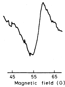
FIG. 1. Field-dependent optogalvanic signal showing the level-crossing B_1^a in the lower ( a^2D_{3/2} ) state of the transition 619.2 nm in ^{89}\text{Y} . Magnetic field modulation. The derivative signal appears on a sloping background, representing the direct effect of the magnetic field on the discharge current. The amplitude of the level-crossing signal represents a change of about 1.5% in the optogalvanic current.
