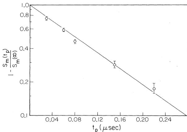
FIG. 2.  $\log[1 - S_m(t_p)/S_m(\infty)]$  vs  $t_p$  for data in Fig. 1. Straight line gives  $\tau = 0.11 \mu\text{sec}$ .
