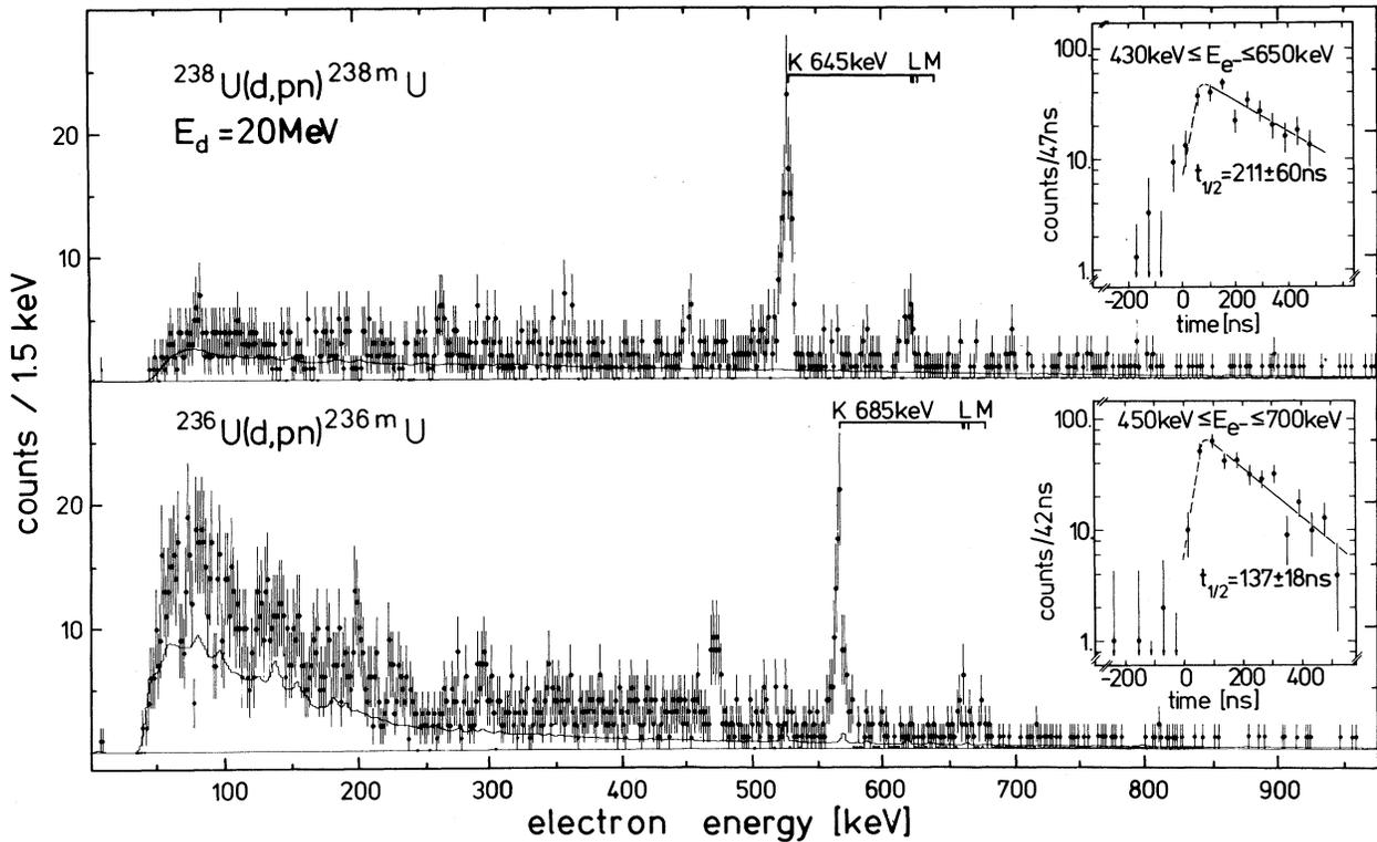
FIG. 2. Energy spectra of electrons in coincidence with the delayed fission decay of the shape isomers  $^{236,238}\text{U}$ . Insets: time spectra of the coincidences for the specified region of electron energies.
