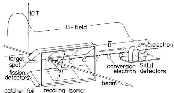
FIG. 1. Experimental setup in the solenoid spectrometer.
