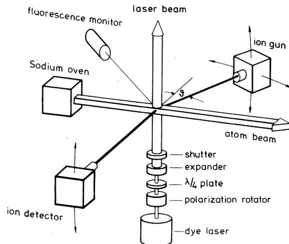
FIG. 1. Schematic diagram of the apparatus.
