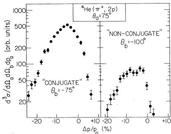
FIG. 1. Momentum spectra of protons detected with the magnet at  $75^\circ$  and 165-MeV  $\pi^+$  incident on a  $^4\text{He}$  target. The left-hand curve is for coincidences with a scintillator at  $-75^\circ$  (the conjugate angle for  $\pi + d \rightarrow 2p$ ) and the right-hand curve for another identical scintillator at  $\theta = -100^\circ$ . The two sets of data are presented with the correct relative normalization.
