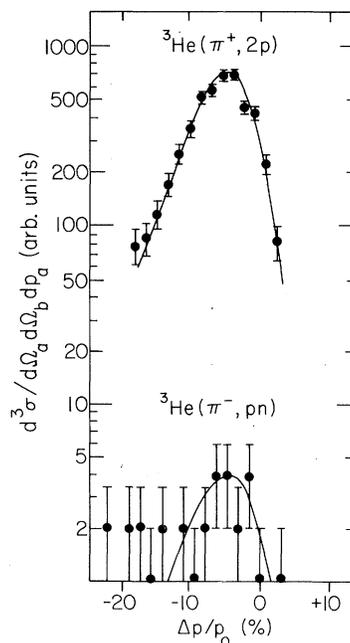
FIG. 2. Momentum spectra of protons detected with the magnet at  $55^\circ$  with 165-MeV pions incident on a  $^3\text{He}$  target. The upper curve was taken with  $\pi^+$  and protons in coincidence in a scintillation arm at  $-100^\circ$ ; while the lower curve is with  $\pi^-$  and neutrons in coincidence. The two sets of data are presented with the correct relative normalization.
