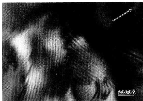
FIG. 1. Electron micrograph showing the structure of the striped-domain phase taken at a temperature of 100 K on warming. The direction of the imaging CDW wave vector is also shown. The micrograph was taken with an exposure time of 30 sec.
