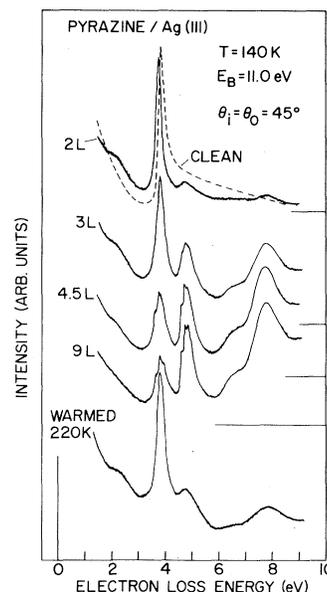
FIG. 1. Electronic-energy-loss spectra for clean Ag(111) and as a function of pyrazine exposure. Specular scattering conditions are used with an elastic beam full width at half maximum of 30 mV.
