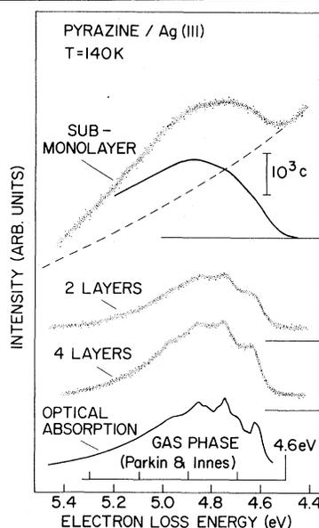
FIG. 2. Electronic-energy-loss spectra for the  ${}^1B_{2u}$  state of monolayer and subsequent adsorbed layers. The optical absorption spectrum for gas-phase pyrazine (Ref. 11) is also shown.
