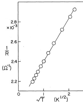
FIG. 3.  $1/R$  vs  $\sqrt{T}$  at a field of 9.2 T for specimen 8.
