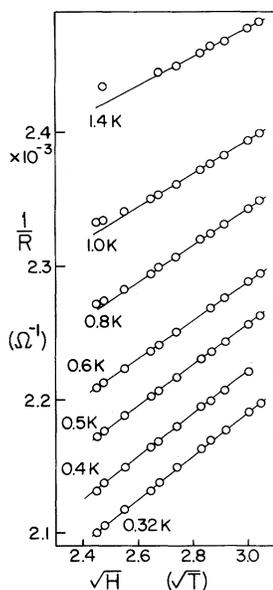
FIG. 1.  $1/R$  vs  $\sqrt{H}$  for specimen 8.  $\rho_{RT} = 8 \times 10^{-3} \Omega \text{ cm}$ .
