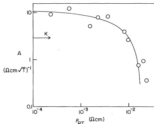
FIG. 2. Log-log plot of  $A \equiv d\sigma/d\sqrt{H}$  as a function of the room-temperature resistivity  $\rho_{RT}$ .
