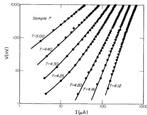
FIG. 3. A logarithmic plot of the current-voltage characteristics of sample 7 at temperatures spanning the critical region  $T_c < T < T_c^0$ . For this sample,  $T_c = 4.16$  K and  $T_c^0 = 4.40$  K. At  $T_c^0$  the  $I$ - $V$  curve is approximately linear, while at  $T_c$ ,  $V$  increases as  $I^3$ .
