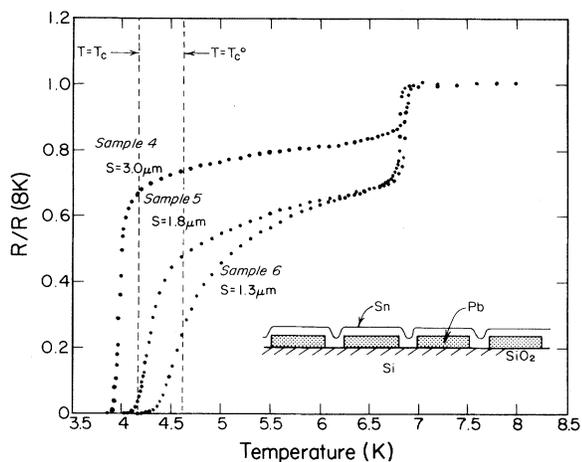
FIG. 1. The temperature dependence of the normalized resistance for samples 4, 5, and 6. The vertical dashed lines mark the values of  $T_c$  and  $T_c^0$  for sample 6. A schematic drawing of the sample construction is illustrated in the inset.
