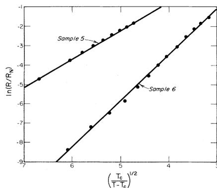
FIG. 2. A logarithmic plot of the resistance of samples 5 and 6 in the temperature range  $T_c < T < T_c^0$ . The data are plotted as a function of the reduced temperature variable  $t^{1/2} = [T_c/(T - T_c)]^{1/2}$ . For sample 5,  $T_c = 4.07$  K while for sample 6,  $T_c = 4.25$  K.
