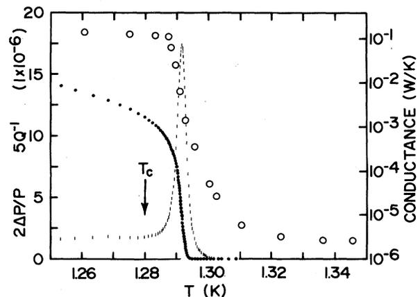
FIG. 2. The period shift  $2\Delta P/P$  (closed circles) and dissipation  $Q^{-1}$  (vertical bars) of the torsional oscillator shown with the total cell conductance (open circles). The  $T_c$  indicated is obtained from fits to the oscillator data.
