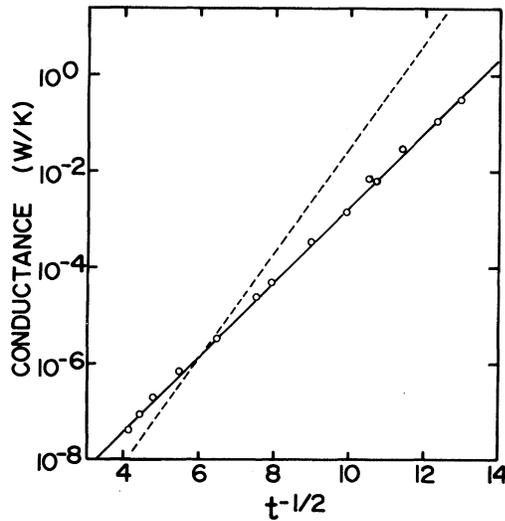
FIG. 3. The conductance  $K_{\text{film}}$  plotted as a function of  $t^{-1/2}$  with  $T_c = 1.2794$  K. The solid line is the fit to the data as discussed in the text. The dashed line represents the film conductance calculated from the parameters obtained from the oscillator data.
