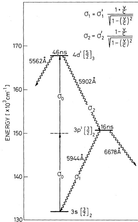
FIG. 2. Reduced energy-level diagram of Ne I showing the harmonic three-level system studied. Also shown is the relativistic transformation, which will locate the two-photon resonance at  $(v_0, \sigma_0)$ , where  $\sigma_0 = \sigma'_1 = \sigma'_2$ .
