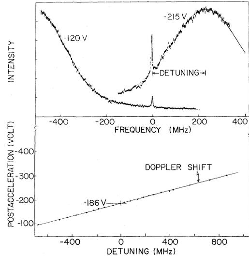
FIG. 4. Experimentally obtained signal seen in the decay  $3p'-3s$  at  $6677 \text{ \AA}$  (upper part). Within our experimental accuracy, the energy separation between the two-photon and the Doppler-broadened resonance ("detuning") arises solely from the Doppler shift, indicating no ac Stark shift of the  $3p'$  level (lower part).
