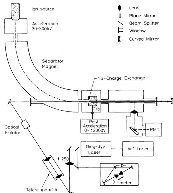
FIG. 1. Experimental apparatus consisting of a 300-kV isotope separator equipped with universal ion source and postacceleration in connection with the charge exchange. Also shown is the stabilized dye laser and  $\lambda$  meter.
