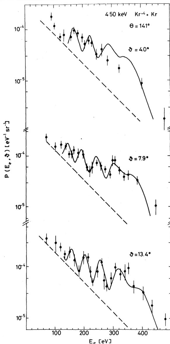
FIG. 1. Electron emission probability as a function of the electron energy  $E_e$  in 450-keV  $\text{Kr}^{+4} + \text{Kr}$  collisions at  $4.0^\circ$ ,  $7.9^\circ$ , and  $13.4^\circ$  laboratory scattering angles under  $141^\circ$  observation angle. The solid lines give the calculated emission probability from a superposition of the background of  $\delta$  electrons (dashed lines) and of the molecular autoionization [Eqs. (1) - (3)].
