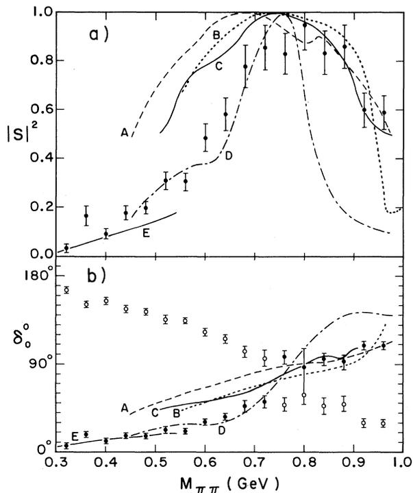
FIG. 4. (a) Extrapolated  $S$ -wave intensity as a function of  $\pi^0\pi^0$  mass. Shown as smooth curves are predictions based on  $\pi^+\pi^-\rightarrow\pi^+\pi^-$  scattering (A and D from Ref. 2, B from Ref. 5, and C from Ref. 4) and on current algebra and partial conservation of axial-vector current (curve E). (b)  $I=0$ ,  $S$ -wave phase shifts determined in our experiment. The two ambiguous solutions are shown as open and closed circles. The curves are as in (a).
