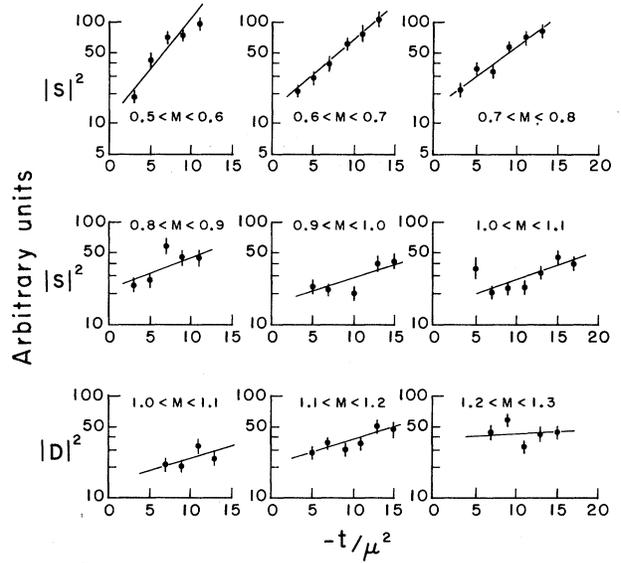
FIG. 3.  $|S|^2$  and  $|D|^2$  as a function of  $t$  for the various  $\pi^0\pi^0$  mass intervals indicated. The straight lines are fits to the data used to obtain the extrapolated amplitudes.
