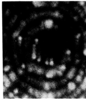
FIG. 5. A field-ion image of growth defects in an ad-layer.
