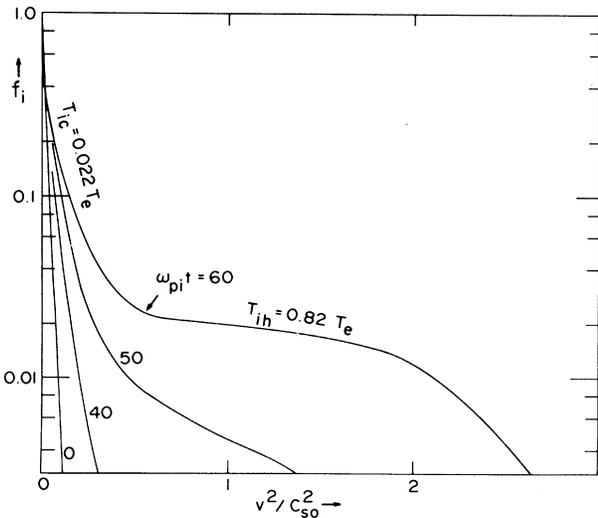
FIG. 1. Time development of ion energy distribution.  $M/m = 1836$ ,  $(T_i/T_e)_{t=0} = 0.01$ ,  $V_d = 0.2(2T_{e0}/m)^{1/2}$ , and  $W(0)/nT_{e0} = 10^{-5}$ .
