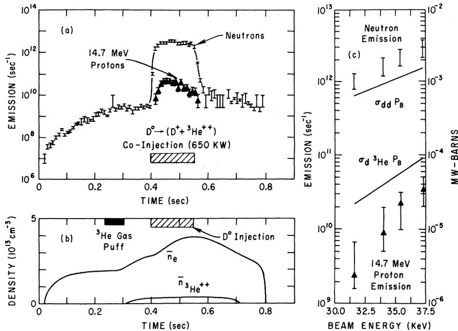
FIG. 2. (a) Time evolution of the 2.5-MeV neutron emission and the 14.7-MeV proton emission during 650-kW deuterium neutral beam injection into a deuterium and <sup>3</sup>He plasma. (b) Time evolution of the line-averaged electron density and <sup>3</sup>He density. (c) Variation of the 2.5-MeV neutron emission and the 14.7-MeV proton emission with neutral beam energy, together with the variation of the respective cross sections weighted with beam power.
