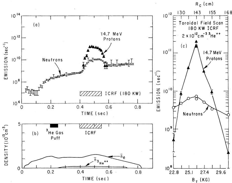
FIG. 3. (a) Time evolution of the 2.5-MeV neutron emission and 14.7-MeV proton emission during 180 kW, 24.6 MHz ICRF heating. (b) Time evolution of the line-averaged electron density and <sup>3</sup>He density. (c) Variation of the 2.5-MeV neutron emission and 14.7-MeV proton emission with the central toroidal magnetic field and therefore with the major radius ( $R_c$ ) of the <sup>3</sup>He<sup>++</sup> cyclotron layer.
