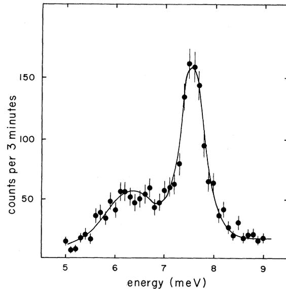
FIG. 3. Zone-boundary phonons, measured at  $Q = (0, 0, 4.5)$ . Incident energy for this scan was 14.7 meV. The collimations from reactor to detector were  $30^\circ-12^\circ-24^\circ-40^\circ$ .
