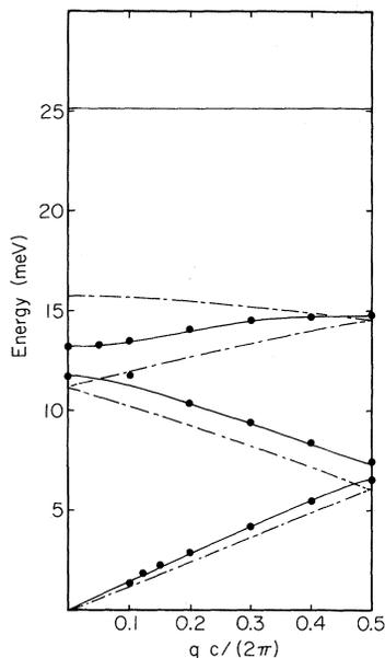
FIG. 2. Dots represent measured phonon energies for [001] L modes in  $C_{36}K$  at 300 K. The phonon dispersion as calculated by a linear chain is given by full lines. The dash-dotted lines show the phonon energies in pure graphite (Refs. 9 and 12). For details, see text.
