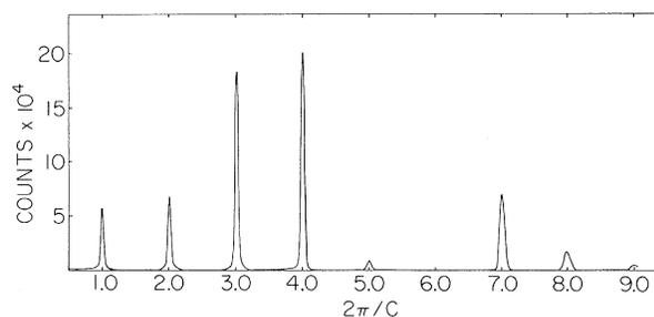
FIG. 1. Elastic (00 $l$ ) scan, measured at 300 K.
