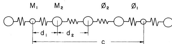
FIG. 4. Linear chain model for (001) L phonons in  $C_{36}K$ .  $a_1 = 2.68$  Å and  $a_2 = 3.35$  Å are the distances between C-K planes and C-C planes, respectively.  $c = 12.07$  Å is the repeat distance in  $C_{36}K$ , disregarding any stacking.
