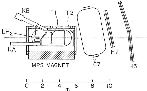
FIG. 1. Schematic diagram of the experimental layout.  $T_1$  and  $T_2$  are planar PWC's;  $H_7$  and  $H_5$  are scintillation-counter hodoscopes;  $C_7$  is the high-pressure Čerenkov counter. All these elements have been used in the triggers. KA and KB are slow  $K^+$  detectors not used in this experiment. The MPS magnet was set at 0.5 T (the direction of the field points into the paper).
