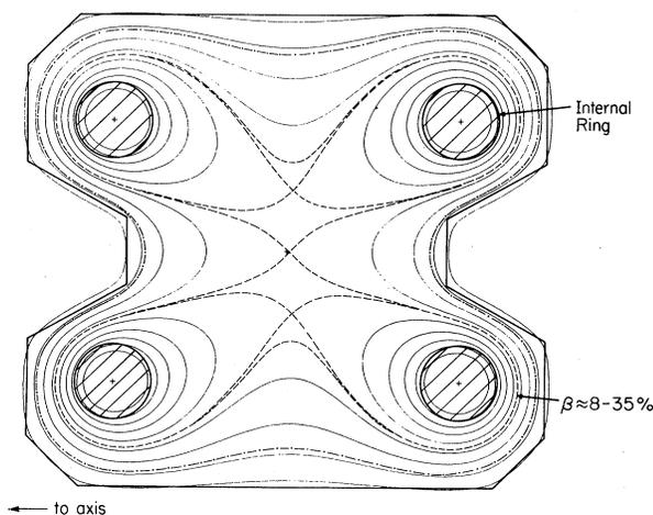
FIG. 1. Poloidal magnetic flux plot of the Levitated Octupole, indicating the bad-curvature region where  $\beta$  is evaluated. Plasma pressure peaks on the separatrix (dashed line). Major radius = 1.4 m.
