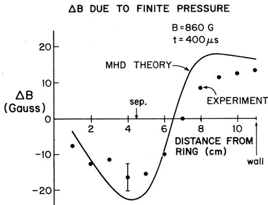
FIG. 2. Single-fluid theoretical and experimental spatial profile (between outer ring and wall) of perturbation,  $\Delta B$ , to the poloidal magnetic field due to the equilibrium diamagnetic currents for  $\beta \approx 8\%$ . Plasma pressure peaks at the separatrix (Sep). Typical error bar is shown.
