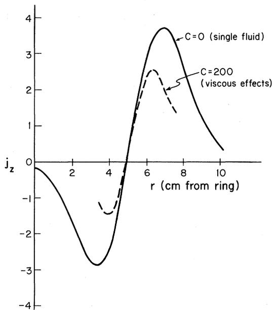
FIG. 4. Spatial profile of the equilibrium current density for the coaxial model of the Octupole from ideal single-fluid theory and viscous two-fluid theory. The two-fluid theory is not plotted near the boundary region where the method of solution breaks down. A Gaussian pressure profile is assumed.
