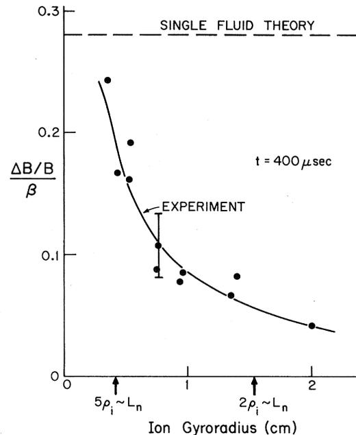
FIG. 3. Theoretical and experimental fractional change in the magnetic field (at the separatrix in the bad-curvature region) due to plasma diamagnetic currents vs thermal ion gyroradius.  $\Delta B/B$  is normalized to the separatrix  $\beta$  value so that single-fluid theory yields a horizontal line.
