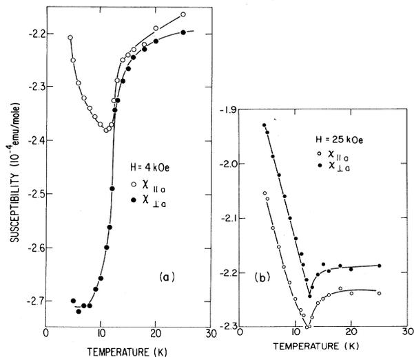
FIG. 1. Static magnetic susceptibility of  $(\text{TMTSF})_2\text{-PF}_6$  parallel and perpendicular to the stacking axis for two different fields, (a) 4 kOe and (b) 25 kOe.
