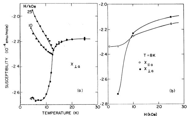
FIG. 2. Evidence for spin flop in  $(\text{TMTSF})_2\text{-PF}_6$ . (a)  $\chi_{\perp a}$  vs  $T$  at 4, 10, and 25 kOe. (b)  $\chi_{\perp a}$  and  $\chi_{\parallel a}$  vs  $H$  at 8 K.
