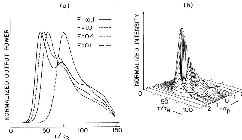
FIG. 2. Influence of diffraction on SF pulse shapes. Parameters are the same as in Fig. 1(a), with  $n_0$  Gaussian and  $\theta_0$  uniform. (a) Emitted power; (b) isometric graph of intensity for the  $F=1$  case of (a).
