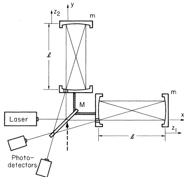
FIG. 1. Schematic of Michelson interferometer ( $b=2$ ) described in text.
