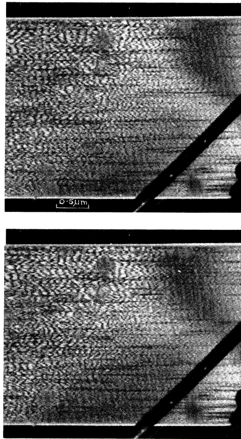
FIG. 1. Images revealing strands parallel to the whisker axis (right-hand sides of the micrographs) and trains of fringes within the strands (left-hand sides). The micrographs were two-second exposures taken with a time interval of approximately one minute. The dark band is the shadow of another whisker.
