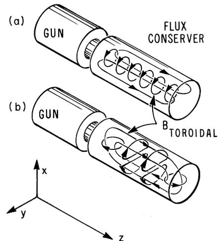
FIG. 1. Schematic of the CT's orientation and shape (a) before and (b) after its major axis rotates by  $90^\circ$ . Note the directions of  $x$ ,  $y$ , and  $z$ .
