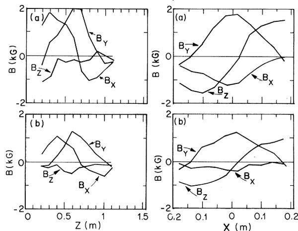
FIG. 5. Magnetic field profiles on the axis and across the midplane of the flux conserver at (a) 25  $\mu s$  and (b) 45  $\mu s$  after the gun is fired. The probe locations are shown in Fig. 4.  $B_y$  is out of the plane of the paper and hence not shown in Fig. 4. It is in the direction of the poloidal field. Axial distance is measured from the gun muzzle.
