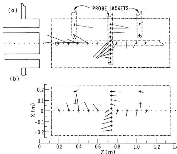
FIG. 4. These typical magnetic-probe data show the toroidal field (a) 5  $\mu s$  and (b) 45  $\mu s$  after the gun is fired. This is the same plane as shown in Fig. 3, but more probes are used here.
