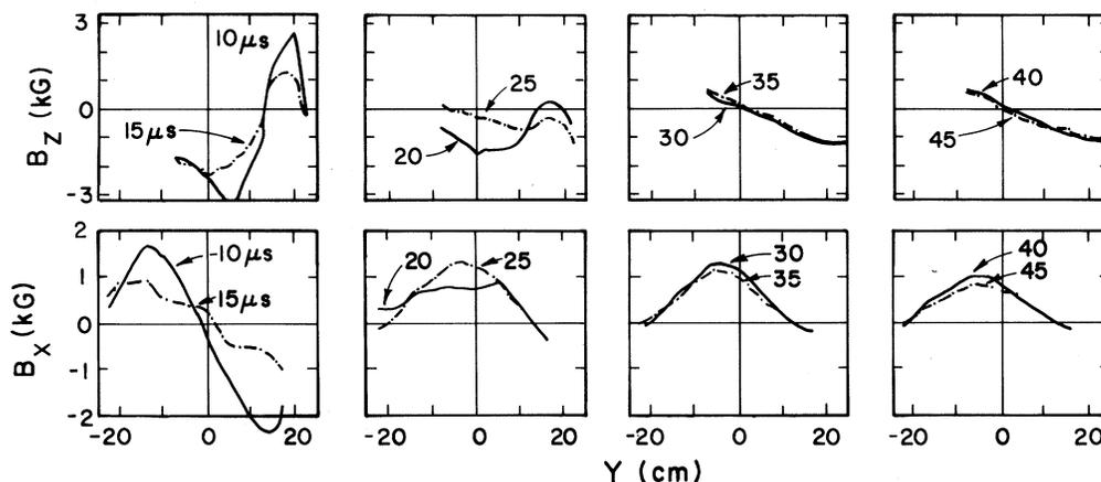
FIG. 2.  $B_x$  and  $B_z$  vs  $y$  at various times. These data are consistent with that produced by a CT which tips as shown in Fig. 1. The data at  $10 \mu s$  correspond to Fig. 1(a) and the data after  $30 \mu s$  correspond to Fig. 1(b). Note that these data are taken  $0.27$  m from the center of the racetrack as shown by the asterisk in Fig. 3.
