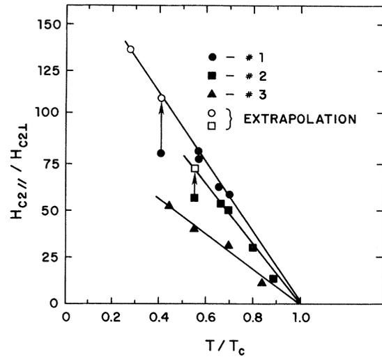
FIG. 3. Upper-critical-field anisotropy,  $H_{c2||}/H_{c2\perp}$ , plotted as a function of reduced temperature. Open points represent extrapolated points because of limitations in the experimental field.
