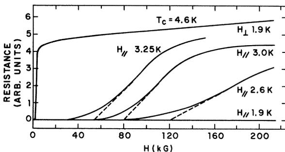
FIG. 1. Resistive transitions induced by applied magnetic fields at selected temperatures.  $H_{c2\parallel}$  has been determined from intercept of dashed lines.
