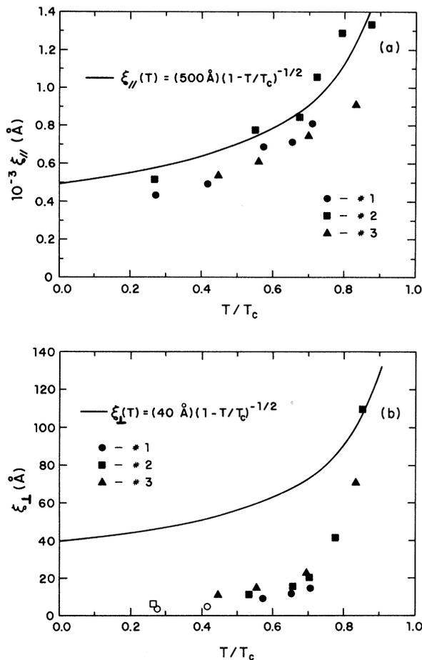
FIG. 4. Temperature dependence of coherence lengths estimated from Eqs. (1) and (2). Solid lines represent GL temperature dependence. (a)  $\xi_{\parallel}$  follows GL fairly closely. (b)  $\xi_{\perp}$  decreases more rapidly than GL and approaches layer spacing below 2 K. Open points are based on extrapolation from Fig. 3.
