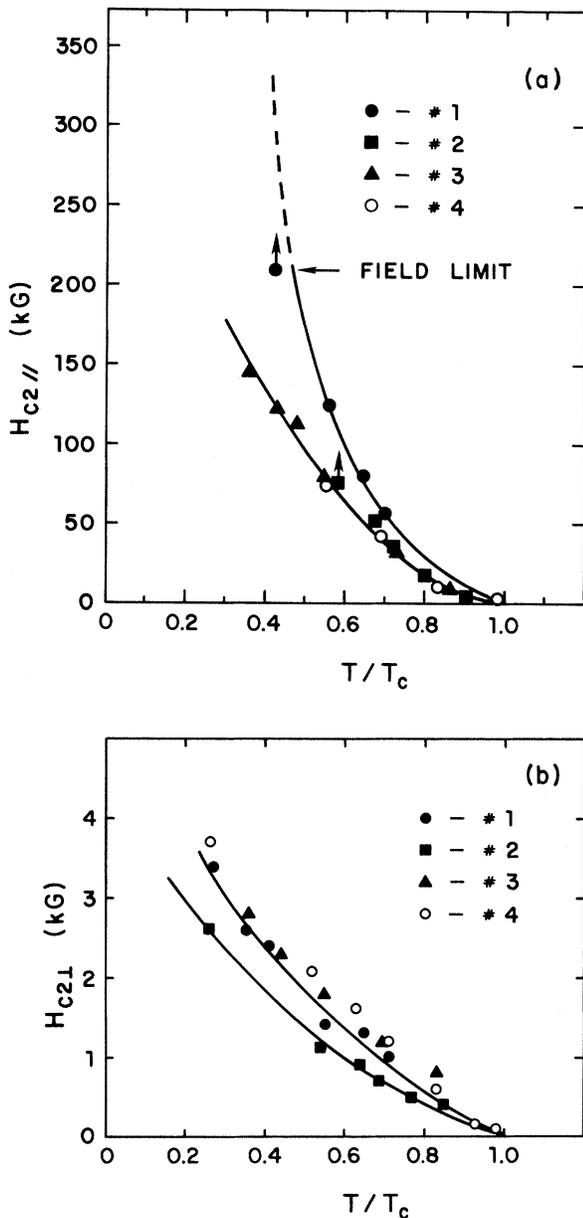
FIG. 2. Upper critical fields (a)  $H_{c2||}$ , (b)  $H_{c2\perp}$  as a function of  $T/T_c$ .  $T_c$ 's for the samples are 4.6 K (No. 1), 4.2 K (No. 2), 3.6 K (No. 3), and 4.1 K (No. 4). Points with arrows are zero resistance at field limit. Dashed line indicates extrapolation based on linear dependence observed in Fig. 3 and the value of  $H_{c2\perp}$ .
