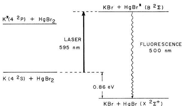
FIG. 1. Schematic diagram of the process being studied. The laser is resonant with neither the reactants nor the products of the reactions. Formation of  $\text{HgBr}^*$  is highly endoergic in the absence of the photon.
