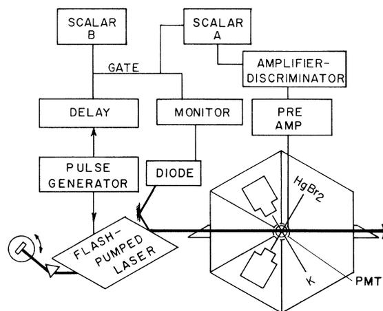
FIG. 2. Experimental apparatus. The light collecting telescope, filter, and photomultiplier are situated directly above the beam intersection region.
