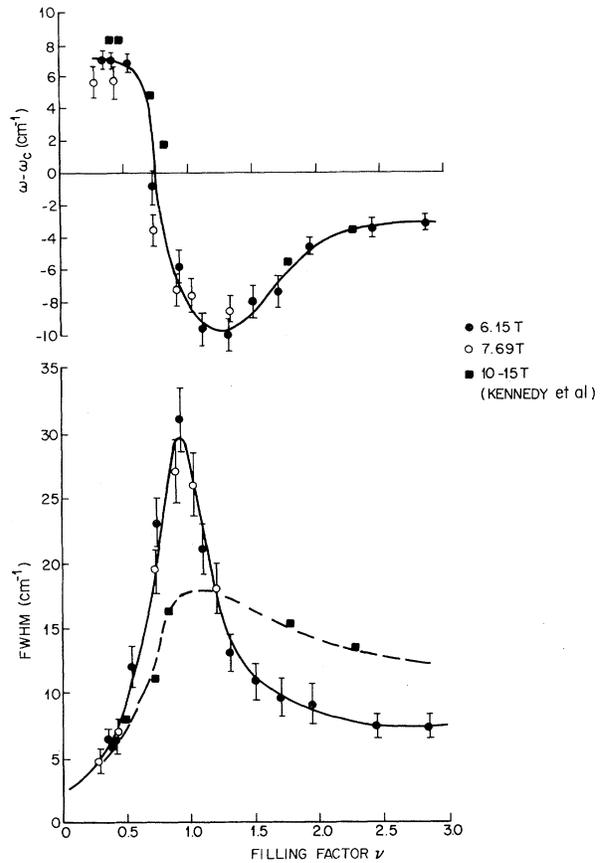
FIG. 2. CR position and width vs filling factor  $\nu$ . Data published by Kennedy *et al.* (Ref. 14) are shown as squares, and the larger width at higher  $\nu$  reflects the lower mobility of that sample.
