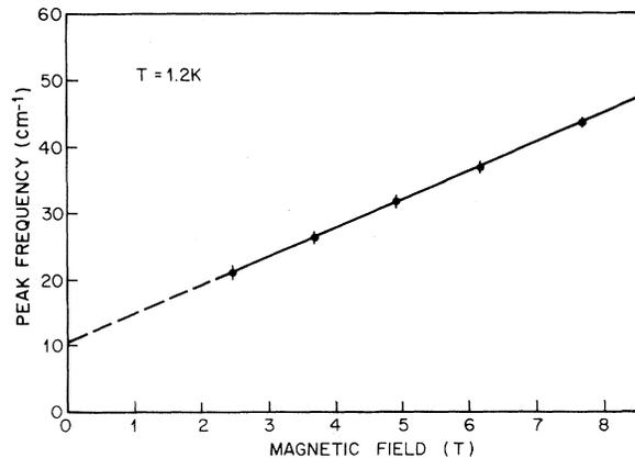
FIG. 3. Position of the CR peak vs magnetic field with  $n_s$  adjusted to maintain  $\nu \approx 0.5$ .
