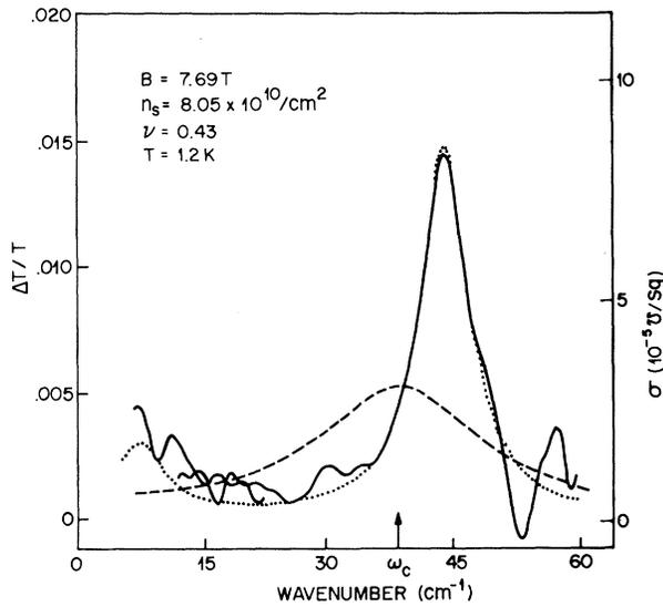
FIG. 1. Cyclotron resonance in the extreme quantum limit. The solid lines represent raw data; the structure is residual noise. The expected classical line shape is shown as a dashed line. The dotted line is a theoretical calculation of the frequency response of a pinned CDW with  $m^* = 0.21m_e$  and a pinning frequency  $\gamma = 20.2 \text{ cm}^{-1}$ , following Ref. 26.
