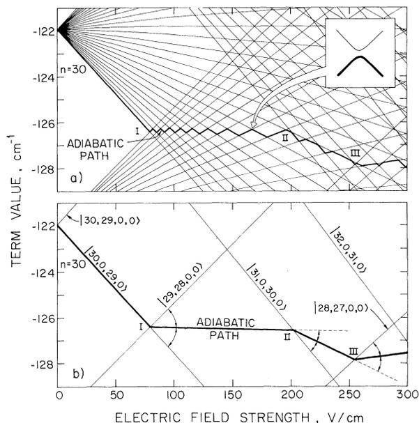
FIG. 2. (a) Schematic representation of the adiabatic path taken by the lowest member of the  $|m_l|=0$  Stark manifold for  $n=30$ . Inset shows the nature of adiabatic crossing. (b) Geometric construction, described in text, to approximate adiabatic path.
