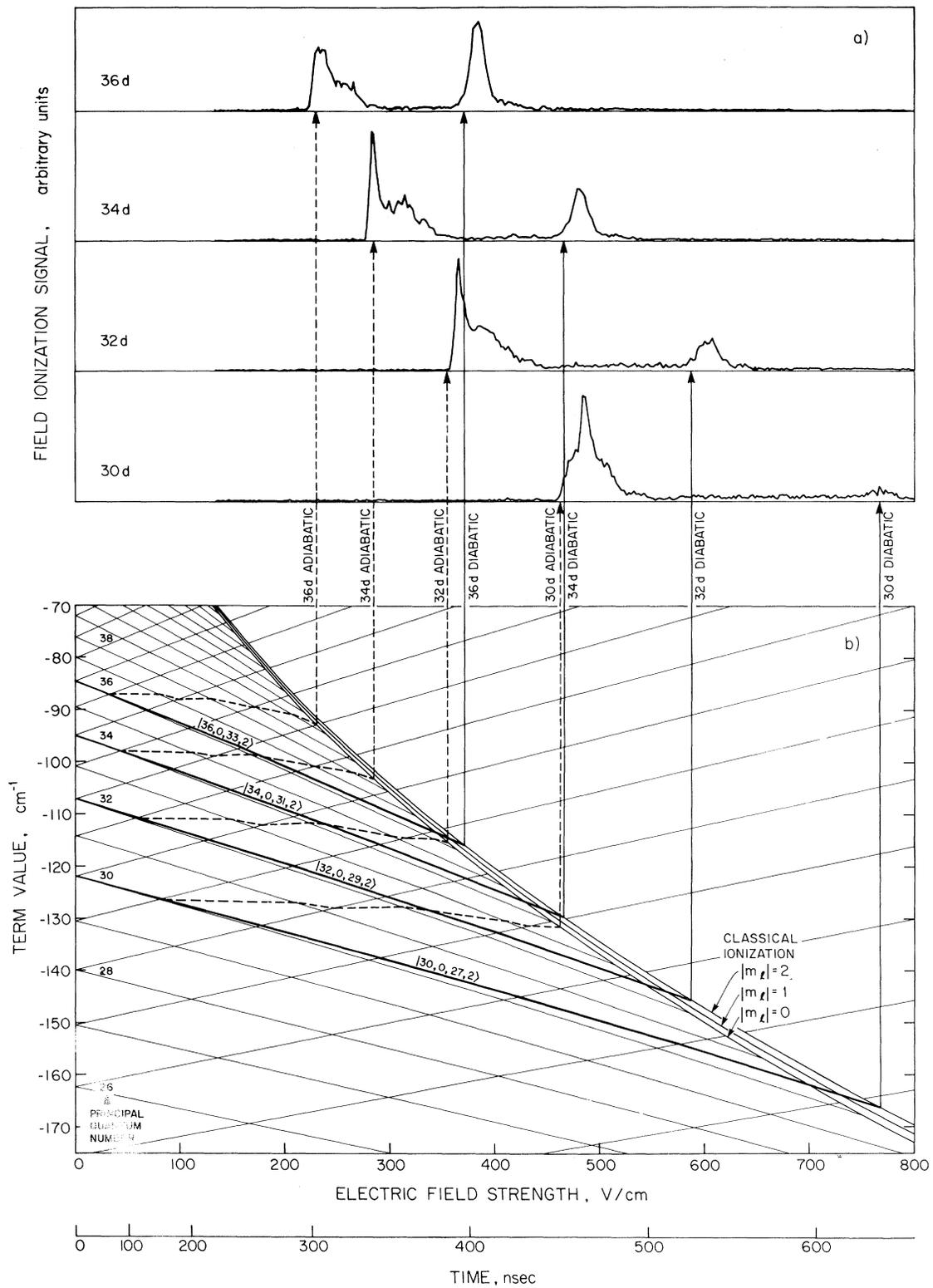
FIG. 1. (a) Field ionization data for  $d$  states of  $n=30, 32, 34,$  and  $36$ . (b) Light lines: extreme members of  $|m_l|=0$  Stark manifolds (fourth order perturbation theory); dotted lines: adiabatic paths to ionization for  $n=30, 32, 34,$  and  $36$ ; dark lines: diabatic paths to ionization for lowest members of  $|m_l|=2$  manifolds for  $n=30, 32, 34,$  and  $36$ . Classical ionization lines calculated on the basis of Ref. 5.
