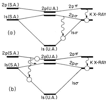
FIG. 1. Schematic correlation diagrams showing (a) the cascade relationship between  $2p\sigma \rightarrow 1s\sigma$  MO transitions and SA  $K$  x rays. (b) Also shown are the effects of rotational coupling which may lead to  $(2p\pi \rightarrow 1s\sigma, K$  x ray) cascades if  $1s\sigma$  vacancies are present in the incoming part of the collision, as in two-collision MO x-ray production.
