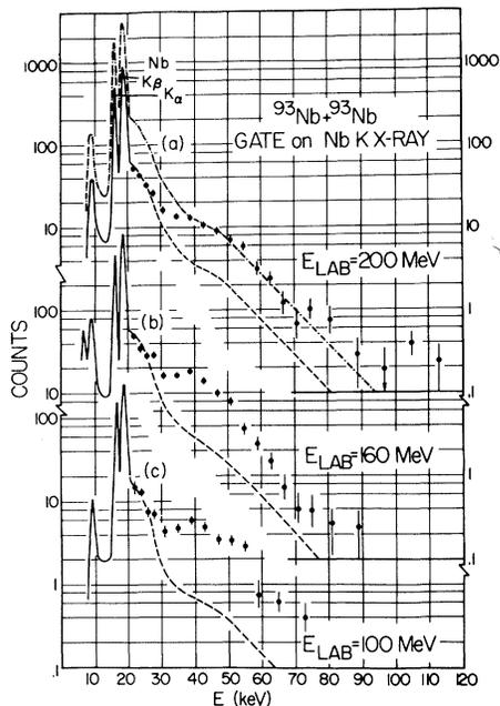
FIG. 2. Solid lines and data points show spectra of x rays in coincidence with SA  $K$  x rays. Solid lines and their continuation into the dashed curves represent singles spectra and reflect contributions to the coincidence spectra from multiple-vacancy processes. Above 30 keV the data have been averaged over twenty channels. The dot-dashed curve in (a) shows the singles spectrum normalized to the coincidence data in the region 40–70 keV.
