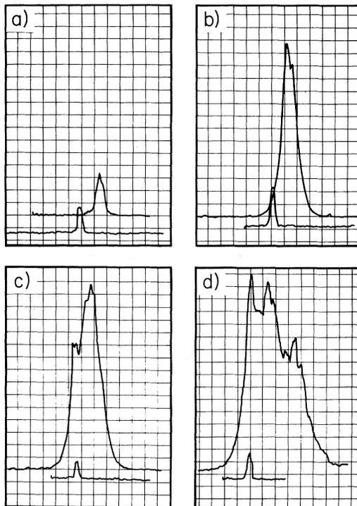
FIG. 2. (a)–(d) Microdensitometer traces of back-reflected spectra. Wavelength increases to the right. Note the location and the spectral width of the incident 1.06- $\mu\text{m}$ -laser energy (the lower traces). The incident power increases from  $2 \times 10^{14} \text{ W/cm}^2$  in (a) to  $2 \times 10^{15} \text{ W/cm}^2$  in (d).
