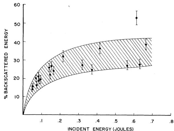
FIG. 3. The total back-reflected energy (Brillouin shifted plus unshifted) as a function of incident laser energy in joules.
