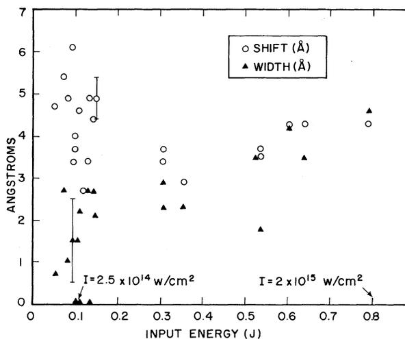
FIG. 4. The measured Brillouin shift and linewidth (FWHM) as a function of incident laser energy.
