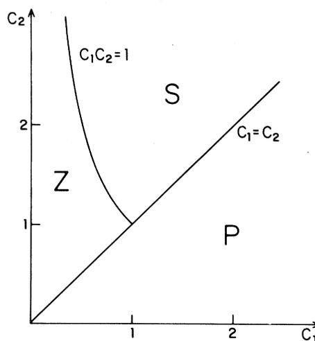
FIG. 1. Regions of stability in the  $c_1, c_2$  plane for the three steady-state solutions.
