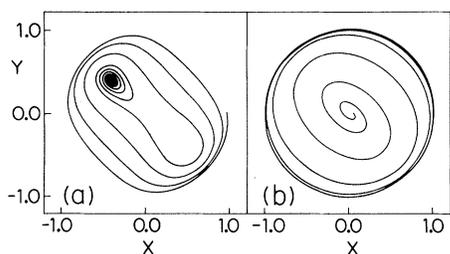
FIG. 2. Trajectories in the  $x$ - $y$  plane for  $c_1 = c_2 = c$ . (a)  $c = 1.5$ . (b)  $c = 0.5$ . Each closed curve represents the solution for a given  $x(0)$ ,  $y(0)$  (or a given value of  $K$ ). The outer circle is solution  $P$ , the center is solution  $Z$ , and the two off-center points in (a) are solution  $S$ . Dotted curve is separatrix.
