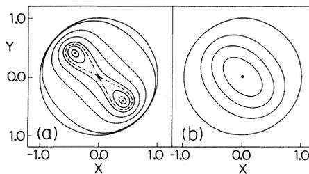
FIG. 3. Trajectories in the  $x$ - $y$  plane for  $c_1 \neq c_2$ . (a)  $c_1 = 1.4$ ,  $c_2 = 1.6$ ,  $x(0) = 0.95$ ,  $y(0) = 0$ . (b)  $c_1 = 0.7$ ,  $c_2 = 0.4$ ,  $x(0) = 0.05$ ,  $y(0) = 0$ .
