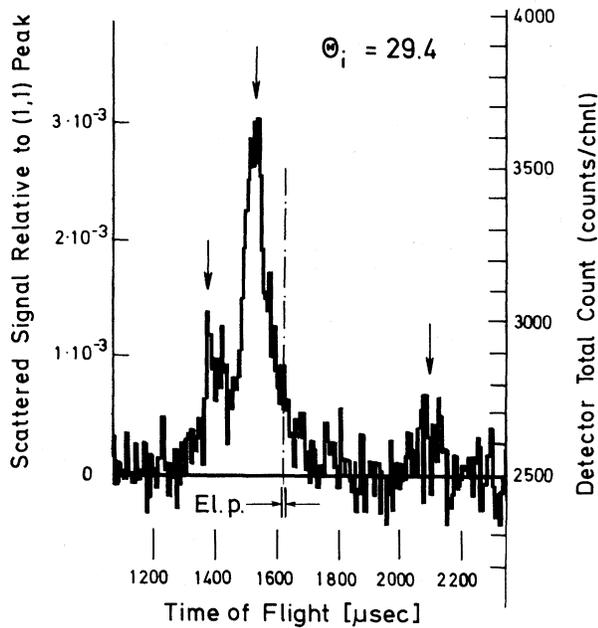
FIG. 1. TOF spectrum for the inelastic scattering of He from the LiF surface ( $6.9 \mu\text{sec}$  channel width, 152 min counting time). The flight time and FWHM of the elastically scattered peak (not present at this incident angle) are indicated.
