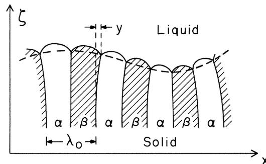
FIG. 1. Schematic illustration of a lamellar eutectic growing up the page with a deformed solidification front. The lamellae may be visualized as semi-infinite plates perpendicular to the plane of the paper. Experiments may also be performed in which the entire sample is a thin film in the plane of the page. The analysis in this paper is most directly applicable to the latter situation.
