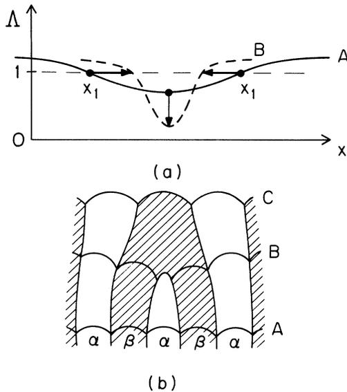
FIG. 2. Schematic illustration of an unstable fluctuation which terminates a lamella. Part (a) shows the function  $\Lambda$  at two successive instants  $A$  and  $B$ . The corresponding sequence of solidification fronts is shown in part (b). Front  $C$  occurs sometime later when the system has restabilized at a larger average value of  $\Lambda$ .
