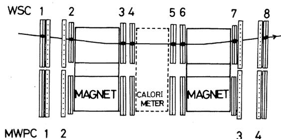
FIG. 1. Schematic view (vertical cross section) of muon spectrometer MUTRON.
