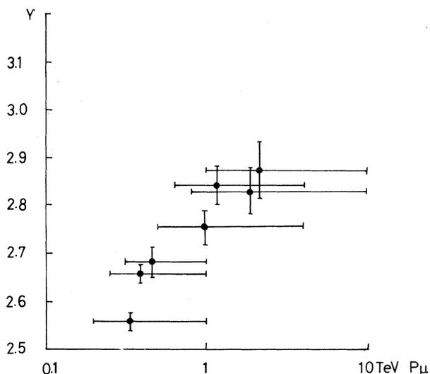
FIG. 2. The  $\gamma$  value of parent mesons at the production. The  $\chi^2$  fits are done over different muon momentum ranges shown by the horizontal bars attached to each datum point.
