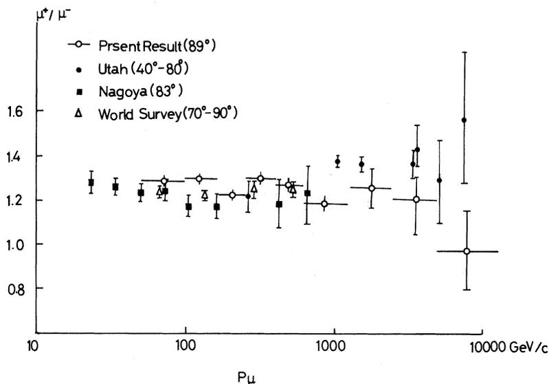
FIG. 3. Muon charge ratio measured by MUTRON (open circles). Previous results of Ahley, Keuffel, and Larson (closed circles; Ref. 15) and of Iida (closed squares; Ref. 14) are presented, together with world survey data of Allkofer, Carsten, Dau, and Jokisch (open triangles; Ref. 14).
