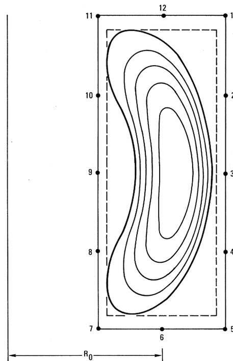
FIG. 1. Geometry used to solve equilibrium problem for  $b/a = 2.5$ .  $H/W$  equilibrium boundary is 300 cm/120 cm;  $R_0 = 145$  cm. Locations where  $\psi$  is specified are labeled like the face of a clock.
