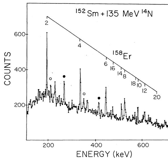
FIG. 3. Spectrum of  $\gamma$  rays coincident with 30–52-MeV tritons. Yrast transitions in  $^{158}\text{Er}$  are labeled with the spin of the initial state.  $\gamma$  rays assigned to  $^{157}\text{Er}$  and  $^{159}\text{Er}$  are marked by closed and open circles, respectively.
