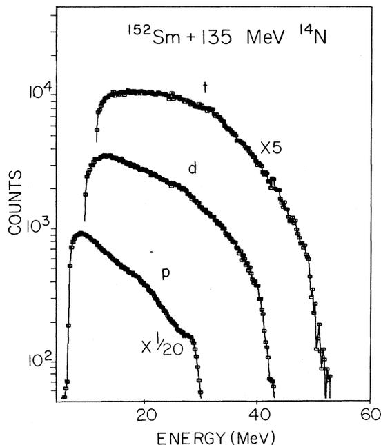
FIG. 2. Proton, deuteron, and triton spectra coincident with any  $\gamma$  ray. The energy scale has not been corrected for the effect of a 54-mg/cm<sup>2</sup> Al absorber.
