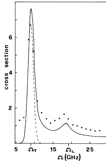
FIG. 2. Brillouin spectrum for (110) GaAs coated with Al. Dots: experimental points. Full line: theoretical cross section. The area under the dashed line indicates the contribution arising from the Rayleigh wave. In this case the reference system has been chosen with the  $x$  axis pointing along the crystallographic [110] direction and the  $z$  axis along the [1 $\bar{1}$ 0] direction.
