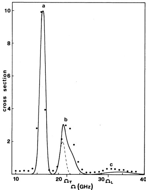
FIG. 1. Brillouin spectrum of (001) Si coated with Al. Dots: experimental points. Full line: theoretical cross section. The area under the dashed line indicates the contribution arising from the second-order Sezawa wave.
