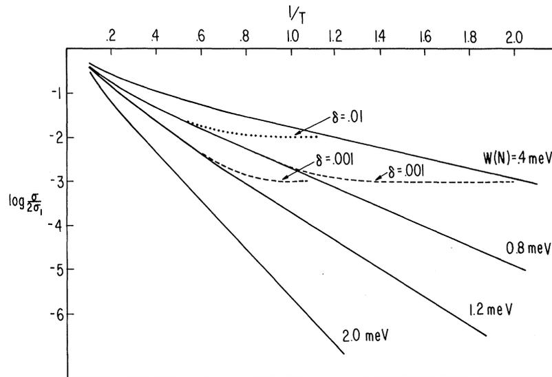
FIG. 2. Plot of the conductivity vs inverse temperature [Eq. (2)] for  $N$  in the activated region.  $W(N)$  is the activation energy in Eq. (1). The solid curves are for  $p = p_c = 0.5$ . The dashed curves are for small deviations,  $\delta = 0.001$ , from  $p_c$ . The dotted curve is for  $\delta = 0.01$ . Note the saturation of the conductivity at low temperature.
