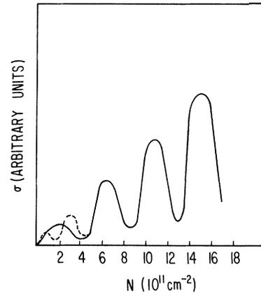
FIG. 3. Sketch of Shubnikov-de Haas oscillations as a function of  $N$  for a magnetic field of 4.4 T. The solid line is the result if no transition occurs. The dashed line shows what happens if the transition occurs at  $N_c \approx 4 \times 10^{11} \text{ cm}^{-2}$ .
