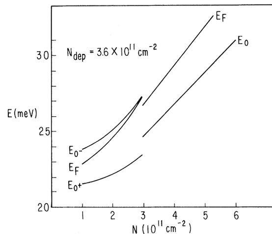
FIG. 1. Results of the density-functional calculation for the lowest subband energy vs density  $N$ . At  $N_c = 2.9 \times 10^{11} \text{ cm}^{-2}$ , there is a first-order phase transition which causes a change in the valley degeneracy.
