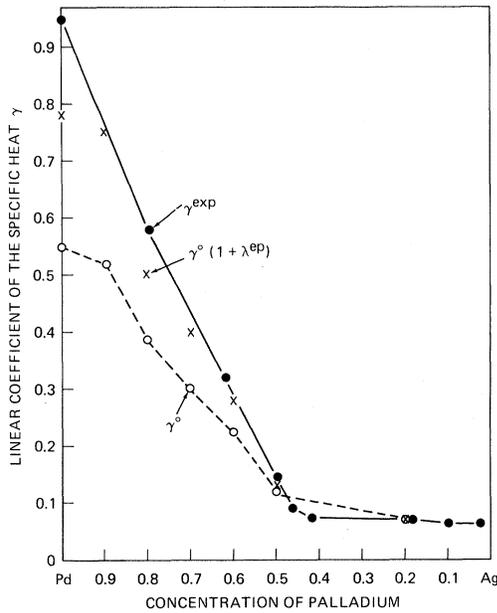
FIG. 1. The linear coefficient of the specific heat vs palladium concentration as calculated from the density of states (open circles), enhanced by the calculated electron-phonon interactions (crosses), and experiments (filled circles).
