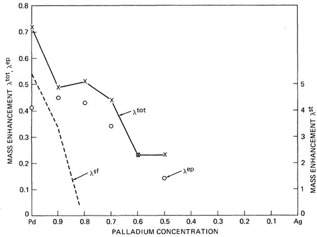
FIG. 2. The total mass enhancement factor  $\lambda^{\text{tot}}$  (crosses), the electron-phonon contribution  $\lambda^{\text{ep}}$  (circles), and the paramagnon contribution of  $\lambda^{\text{SF}}$  (dashed curve) vs palladium concentration.
