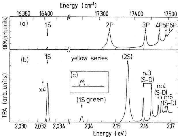
FIG. 1. One- and two-photon spectra of  $\text{Cu}_2\text{O}$ . (a) One-photon data at 4.2 K from Ref. 14. (b) Two-photon data at 4.5 K; the yellow 1S line was measured at 20 K. (c) Splitting of green 1S exciton in a magnetic field of 8.5 T (Voigt configuration). Note the enlarged energy scale for the yellow 1S region.
