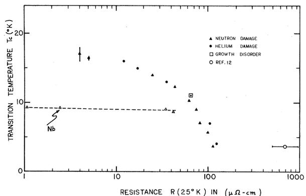
FIG. 1. Superconducting transition temperature of V<sub>3</sub>Si subjected to various types of damage as a function of residual resistivity. The universal drop in  $T_c$  is common to other A-15 compounds, and is in sharp contrast to the behavior of Nb shown by the dotted curve.
