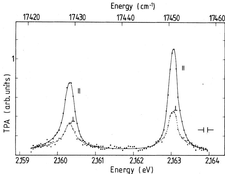
FIG. 2. Two-photon spectra of the  $n=3$  excitons for different polarization configurations at 4.5 K (resolution 0.1 meV). In  $\parallel$  configuration, both polarization vectors  $\vec{\epsilon}_1$  and  $\vec{\epsilon}_2$  are parallel to  $[\bar{1}\bar{1}1]$ ; in  $\perp$  configuration,  $\vec{\epsilon}_1$  in  $[111]$  and  $\vec{\epsilon}_2$  in  $[1\bar{1}2]$  directions.
