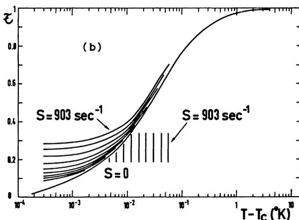
FIG. 1. (a) Scattering geometry.  $O$  is the center of symmetry of the pipe. (b) Transmitted intensity vs  $T - T_c$  at decreasing shear rates  $S = 903, 510, 288, 163, 92, 52, 29, 16, 9.5,$  and  $0 \text{ sec}^{-1}$ . Vertical lines correspond to the crossover temperature where  $S\tau = 1$ .
