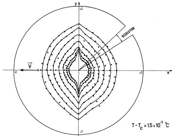
FIG. 3. Reduced intensity  $i$  (see text) in the  $x$ - $y$  plane at constant light wave number  $q_1 = 1.82 \times 10^4 \text{ cm}^{-1}$ ,  $T - T_c = 1.5 \times 10^{-3} \text{ }^\circ\text{C}$  and for decreasing shear rates  $S = 903, 510, 288, 163, 92, 52, 29,$  and  $0 \text{ sec}^{-1}$ . The smallest curve corresponds to  $S = 903 \text{ sec}^{-1}$ , and the circle of radius unity to  $S = 0$ .
