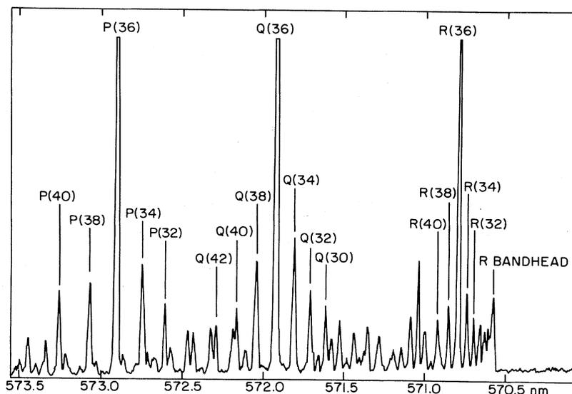
FIG. 2. Optical-optical double-resonance excitation of the  $^1\Pi_g$  ( $\psi = 1$ ) band following pumping of the  $A^1\Sigma_u^+$  ( $\psi = 2$ ,  $J = 36$ ) level of  $^7\text{Li}_2$ . The wavelength scale is the probe-laser wavelength.
