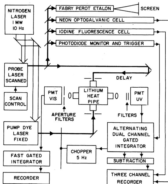
FIG. 1. Schematic diagram of the experimental arrangement for performing pulsed optical-optical double-resonance spectroscopy on  $^7\text{Li}_2$  using ultraviolet fluorescence detection and signal treatment in which spectral features originating from only one of the two dye lasers are subtracted before final recording.
