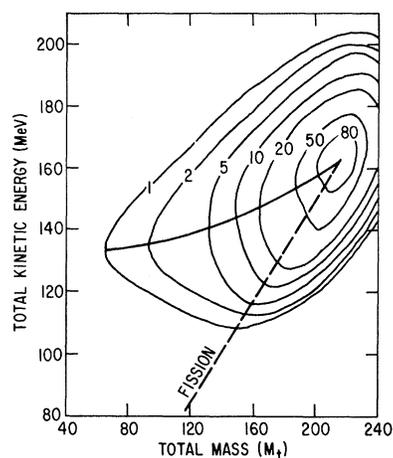
FIG. 3. Contour plot of the correlation between total kinetic energy and total mass of binary fragments. The full line indicates the path of most probable values, the dashed line the relation expected for fission (see text).
