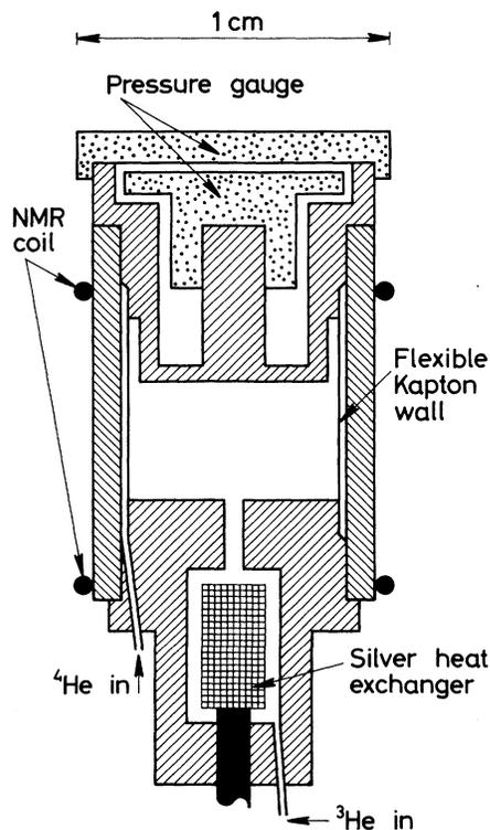
FIG. 1. Pressure cell for NMR detection during compressional cooling of  $^3\text{He}$ .
