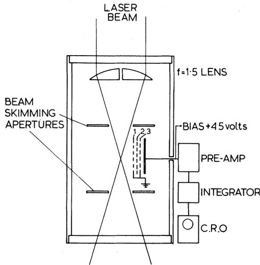
FIG. 1. Experiment with laser focus in vacuum chamber containing helium of pressures  $10^{-6}$  to  $10^{-3}$  Torr. 1, 2, and 3 are grids in front of the probe.
