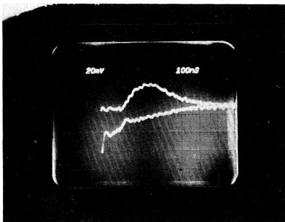
FIG. 2. Probe signal of electron and ion pulses at a pressure of  $8 \times 10^{-3}$  Torr.
