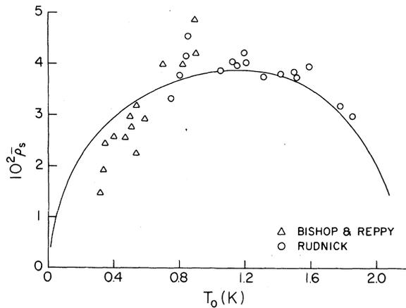
FIG. 4. The effective superfluid density at onset  $\rho_s$  calculated from Eq. (17) and compared with experiments of Rudnick (Ref. 9) and Bishop and Reppy (Ref. 8).
