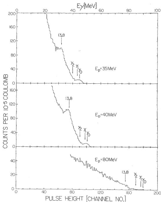
FIG. 2.  $\gamma$ -ray spectra from 35-, 40-, and 60-MeV protons on  $^{27}\text{Al}$  observed at  $60^\circ$ . See Fig. 1 for notation.
